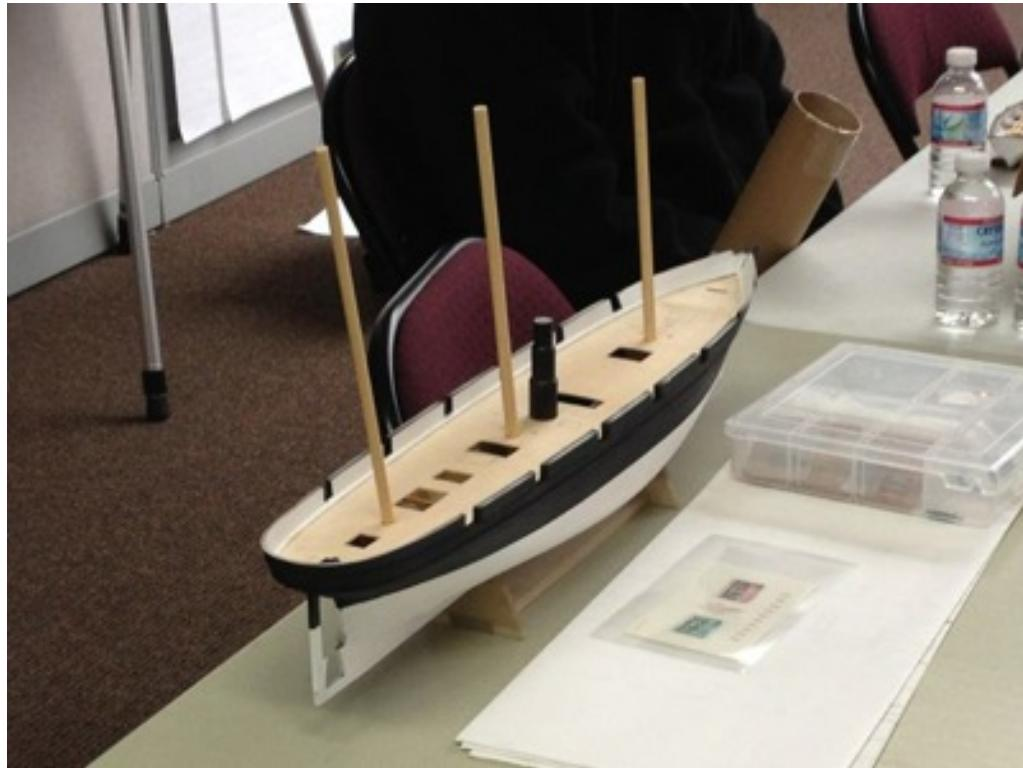
The 1/75-scale model is from a plank-on-bulkhead kit by Woody Joe of Japan, with modifications based on drawings obtained from the Prince Hendrik Museum in Holland.
